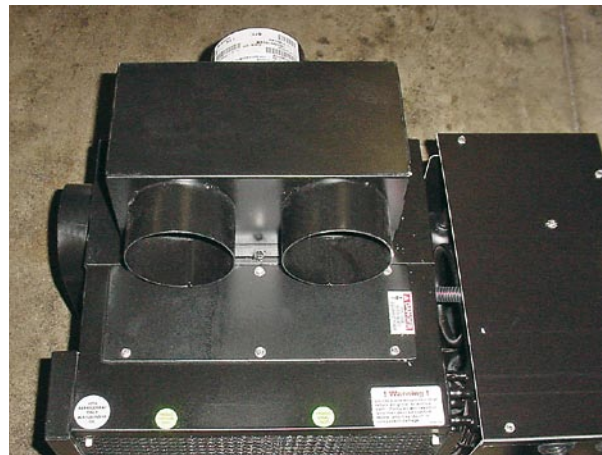
Figure 18b - Installing the air distribution plenum
